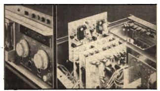
L-Closely grouped audio controls. Potentiometers and push buttons for Input and output level as well as headphones level.
